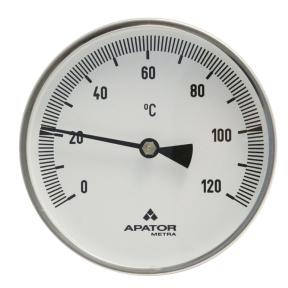
or in liquid environment, stem must be placed in thermometer well. Maximum pressure when well is used is 0,6 MPa. Thermometers TR with stem length 45 and 60 mm and thermometers with range 0  $^{\circ}$ C - 350  $^{\circ}$ C and 0  $^{\circ}$ C - 450  $^{\circ}$ C can be used only with thermometer well.
